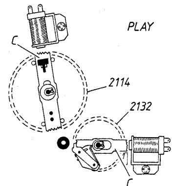
Set the camwheel 2132 in its stop position.
