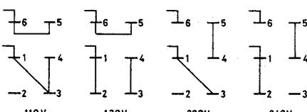
MAINS VOLTAGE CONNECTIONS AND FUSES ARE PLACED
