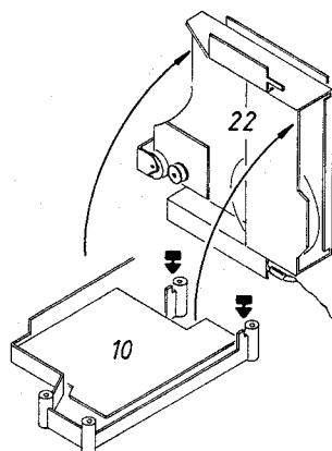
Remove the top plate of the record player and place the radio section in servicing position.
